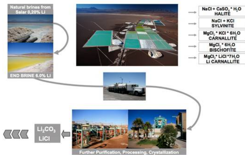
Figure 195: Lithium production process in Chile
