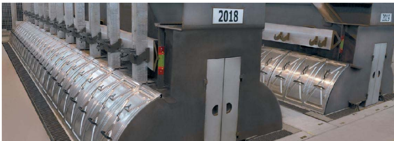
Figure 122: Aluminium smelting cells (or pots) at Rio Tinto's Kitimat smelter in Canada
